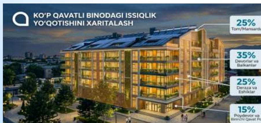
Figure 1. Heat loss map in multi-story buildings
