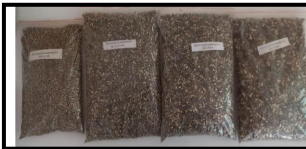
2-pictures. Small and large fractionated vermiculite concentrates in the form of small grains and their bulk samples
